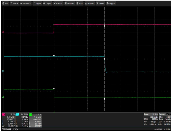
Figure 7: CSV2000BP-3 Turn Off Characteristic via PS_ON Load: I_O = 163.9A I_{SB} = 3.5A Ch 2: PS_ON_L Ch 3: V_O Ch 4: PWOK
