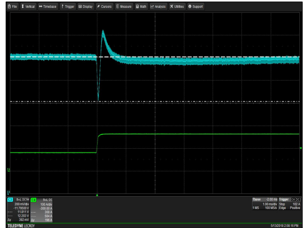
Figure 8: CSV2000BP-3 Transient Response - V_O Deviation 50% to 100% load change 1A/uS slew rate V_{in} = 230Vac Ch 3: V_O Ch 4: I_O
