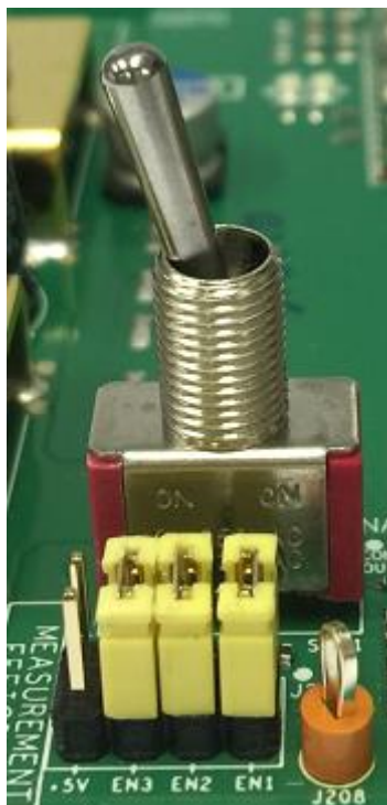
Fig. 4 – Enable jumper location and population
