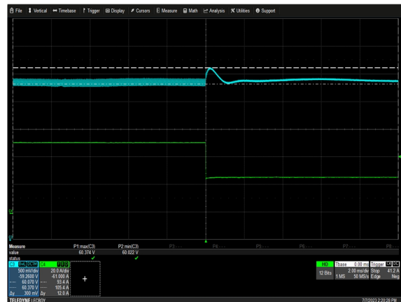
Figure 66: TF3000A60K Transient Response - V_o Deviation 100% to 50% load change 1A/\mu S slew rate V_{IN} = 230Vac Ch 3: V_o Ch 4: I_o
