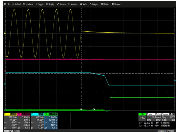
Figure 42: TF3000A48K Hold-up Time V_{IN} = 264\text{Vac} Load: I_o = 62.5\text{A} , V_{AUX} = 5\text{V} , I_{AUX} = 0.5\text{A} Ch 1: V_{IN} Ch 2: V_{AUX} Ch 3: V_o Ch 4: POK
