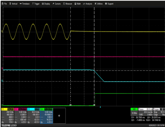
Figure 41: TF3000A48K Hold-up Time V_{IN} = 90\text{Vac} Load: I_o = 31.25\text{A} , V_{AUX} = 5\text{V} , I_{AUX} = 0.5\text{A} Ch 1: V_{IN} Ch 2: V_{AUX} Ch 3: V_o Ch 4: POK
