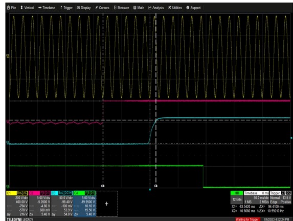
Figure 58: TF3000A60K Turn-on delay via EN V_{IN} = 264\text{Vac} Load: I_o = 50\text{A} , V_{AUX} = 5\text{V} , I_{AUX} = 0.5\text{A} Ch 1: V_{IN} Ch 2: EN Ch 3: V_o Ch 4: POK
