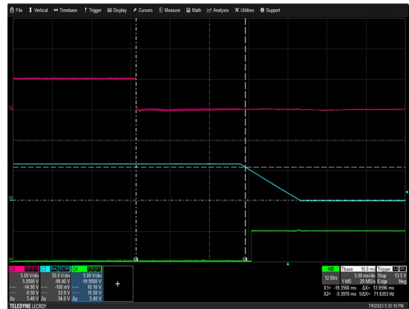
Figure 64: TF3000A60K Turn Off Characteristic via EN V_{IN} = 230Vac Load: I_o = 50A Ch 2: EN Ch 3: V_o Ch 4: POK
