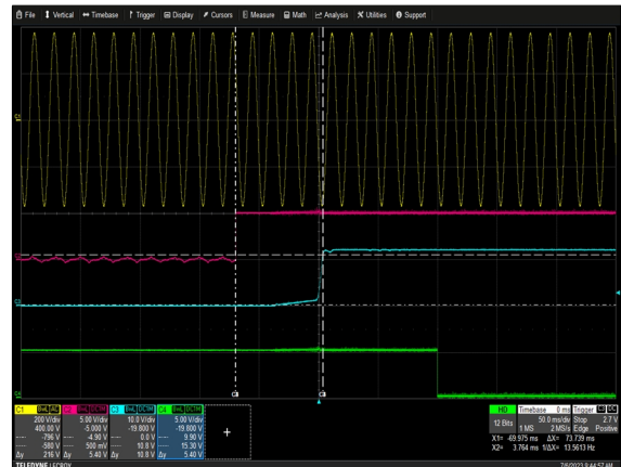
Figure 4: TF3000A12K Turn-on delay via EN V_{IN} = 264\text{Vac} Load: I_o = 200\text{A} , V_{AUX} = 5\text{V} , I_{AUX} = 0.5\text{A} Ch 1: V_{IN} Ch 2: EN Ch 3: V_o Ch 4: POK
