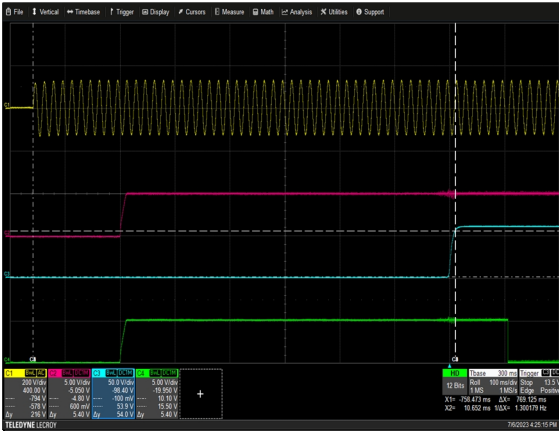
Figure 55: TF3000A60K Turn-on delay via AC mains V_{IN} = 90\text{Vac} Load: I_o = 25\text{A} , V_{AUX} = 5\text{V} , I_{AUX} = 0.5\text{A} Ch 1: V_{IN} Ch 2: V_{AUX} Ch 3: V_o Ch 4: POK
