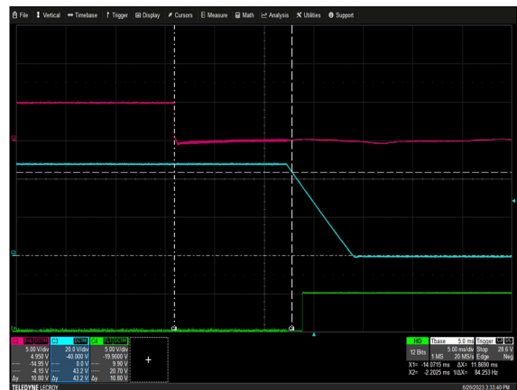
Figure 46: TF3000A48K Turn Off Characteristic via EN V_{IN} = 230Vac Load: I_o = 62.5A Ch 2: EN Ch 3: V_o Ch 4: POK
