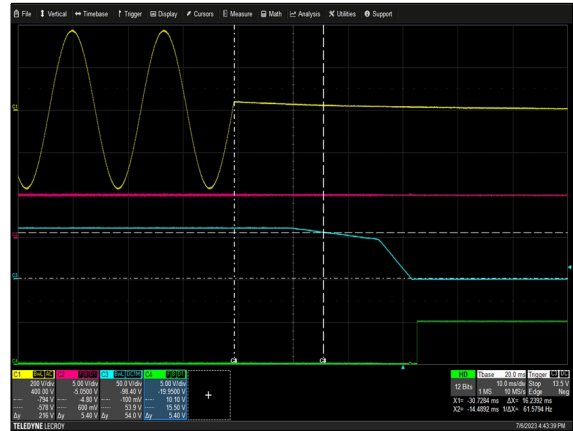
Figure 60: TF3000A60K Hold-up Time V_{IN} = 264\text{Vac} Load: I_o = 50\text{A} , V_{AUX} = 5\text{V} , I_{AUX} = 0.5\text{A} Ch 1: V_{IN} Ch 2: V_{AUX} Ch 3: V_o Ch 4: POK
