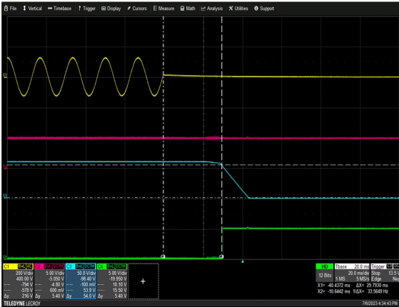
Figure 59: TF3000A60K Hold-up Time V_{IN} = 90\text{Vac} Load: I_o = 25\text{A} , V_{AUX} = 5\text{V} , I_{AUX} = 0.5\text{A} Ch 1: V_{IN} Ch 2: V_{AUX} Ch 3: V_o Ch 4: POK
