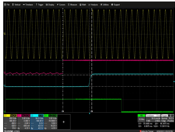
Figure 40: TF3000A48K Turn-on delay via EN V_{IN} = 264\text{Vac} Load: I_o = 62.5\text{A} , V_{AUX} = 5\text{V} , I_{AUX} = 0.5\text{A} Ch 1: V_{IN} Ch 2: EN Ch 3: V_o Ch 4: POK
