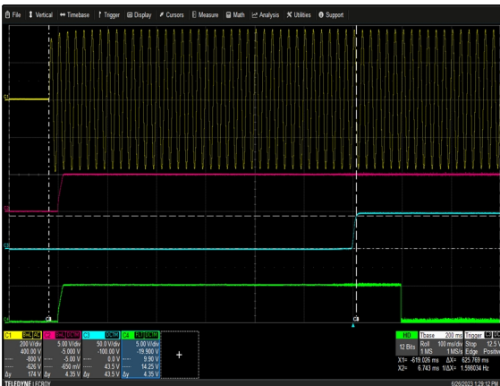
Figure 39: TF3000A48K Turn-on delay via AC mains V_{IN} = 264\text{Vac} Load: I_o = 62.5\text{A} , V_{AUX} = 5\text{V} , I_{AUX} = 0.5\text{A} Ch 1: V_{IN} Ch 2: V_{AUX} Ch 3: V_o Ch 4: POK
