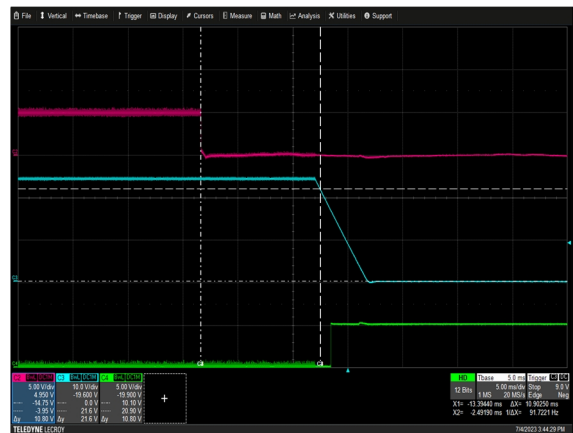
Figure 28: TF3000A24K Turn Off Characteristic via EN V_{IN} = 230V_{ac} Load: I_o = 125A Ch 2: EN Ch 3: V_o Ch 4: POK
