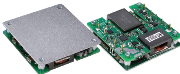
Figure 11: Advanced Energy's Artesyn ADH700, 700 W DC-DC converter, powers GaN RF power amplifiers in a 5G RAN base station
