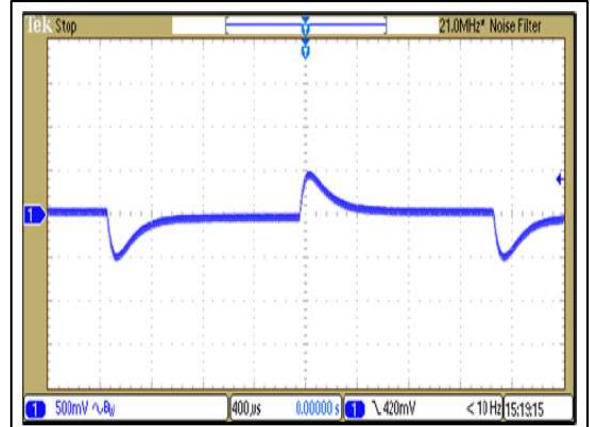
Figure 64: ERM01U100 Transient Response Vin = 110Vdc Load: Io = 100% to 75% load change Ch 1: Vo
