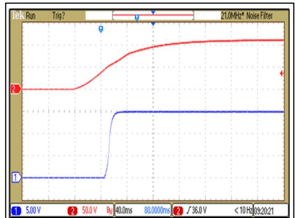
Figure 36: ERM06C100 Output Voltage Startup Characteristic by Vin Vin = 110Vdc Load: Io = 6.7A Ch 1: Vin Ch 2: Vo
