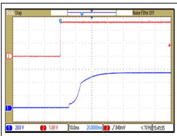
Figure 65: ERM01U100 Output Voltage Startup Characteristic by On/Off Vin = 110Vdc Load: Io = 1.85A Ch 1: Remote On/Off Ch 2: Vo
