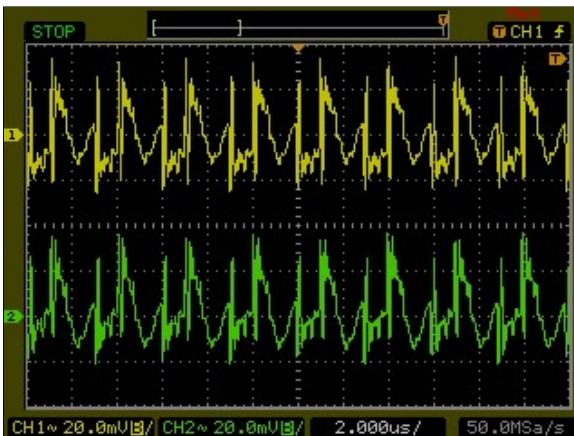
Figure 110: AXA00CC36-L Ripple and Noise Measurement Vin = 48Vdc Load: Io = ±0.67 A Ch 1: Vo
