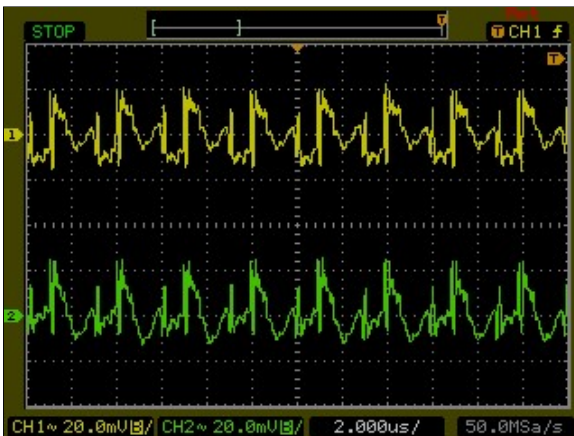
Figure 57: AXA00CC18-L Ripple and Noise Measurement Vin = 24Vdc Load: Io = ±0.67 A Ch 1: Vo1 Ch 2: Vo2
