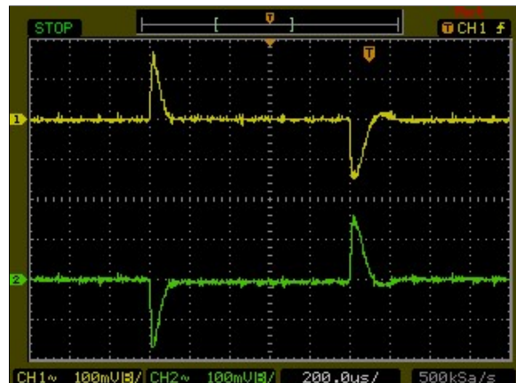
Figure 102: AXA00BB36-L Transient Response Vin = 48Vdc Load: Io = 100% to 75% load change Ch 1: Vo1 Ch2:Vo2
