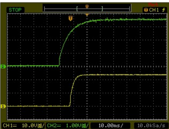
Figure 41: AXA00H18-L Output Voltage Startup Characteristic by ON/OFF Vin = 24Vdc Load: Io = 0.835A Ch1: Vo Ch2: Remote On/Off
