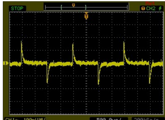
Figure 103: AXA00H36-L Transient Response Vin = 48Vdc Load: Io = 100% to 75% load change Ch 1: Vo
