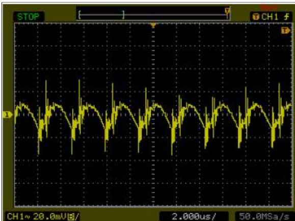
Figure 3: AXA04F18-L Ripple and Noise Measurement Vin = 24Vdc Load: Io = 4.5A Ch 1: Vo
