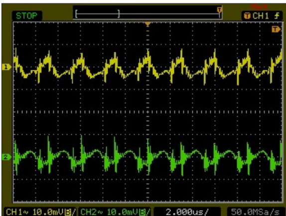
Figure 48: AXA00BB18-L Ripple and Noise Measurement Vin = 24Vdc Load: Io = ±0.835 A Ch 1: Vo1 Ch 2: Vo2
