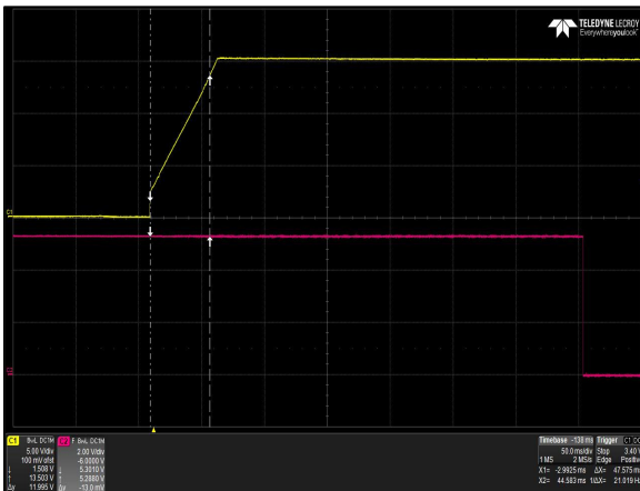
Figure 16: LCM1000N-T-4 Output Voltage Startup Characteristic Vin = 90Vac Load: lo = 66.7A (15V), I SB = 1A (5V) Ch 1: Vo Ch 2: G_DCOK_C
