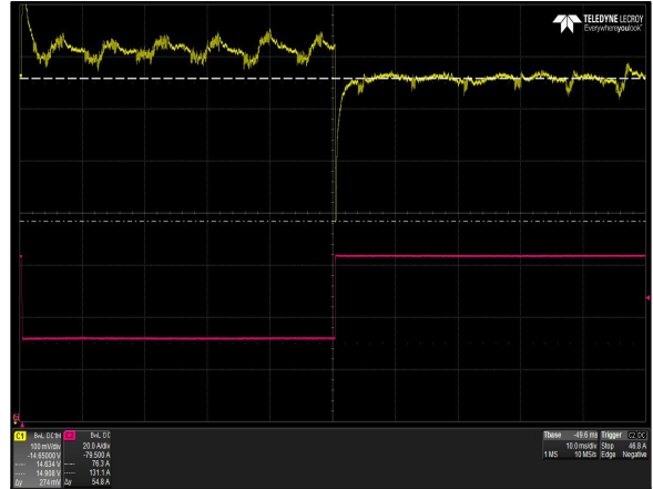
Figure 19: LCM1000N-T-4 Transient Response - Vo Deviation 100% to 50% load change 1A/uS slew rate Vin = 90Vac Ch 1: Vo Ch 2: Io
